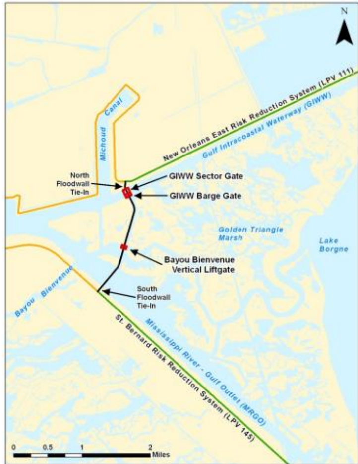
Figure 14: Design of the Inner Harbor Canal-Lake Borgne Surge Barrier
